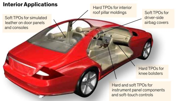
ENGAGE™ polyolefin elastomers have long been the impact modifiers of choice in TPO applications. Today, Dow advances in performance and processability enable production of best-in-class TPOs for interior and exterior molded parts that meet demands for:
